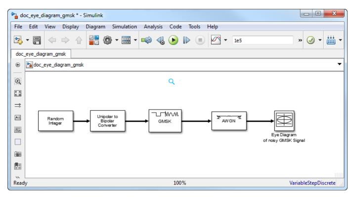
Run the model. The eye diagram is configured to show a histogram without interpolation.
