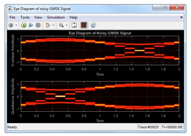
The lack of interpolation results in a plot having piecewise-continuous behavior.
